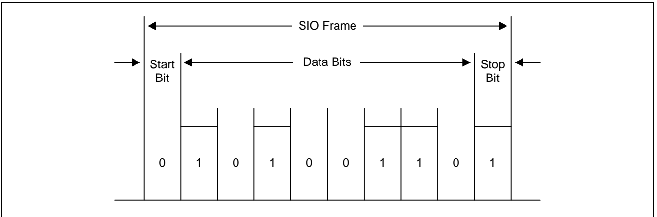
Figure 11-5. Serial I/O Frame Timing Diagram (Normal UART)
